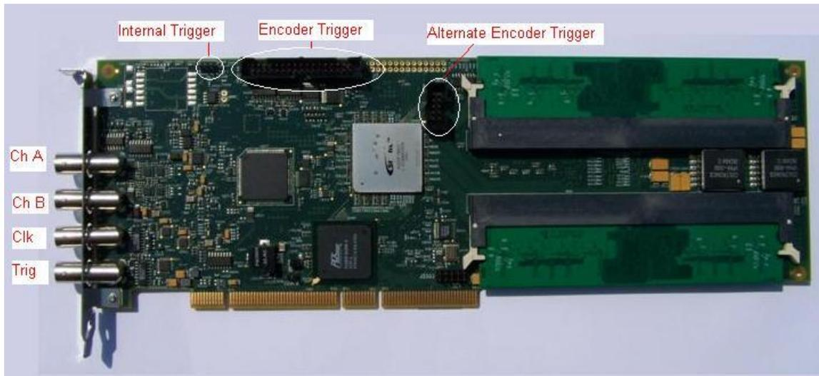
Figure 14: AL8xGT with labeled connectors (front)
