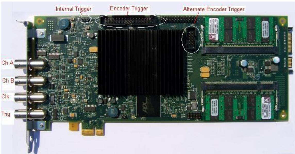
Figure 16: AL8xGT-Express with labeled connectors (front)
