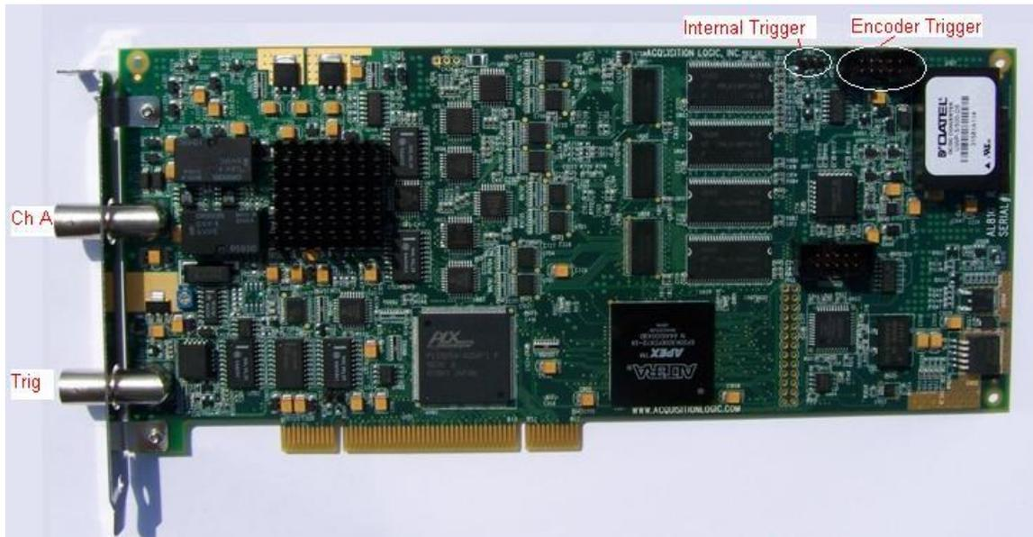
Figure 13: AL81G with labeled connectors
